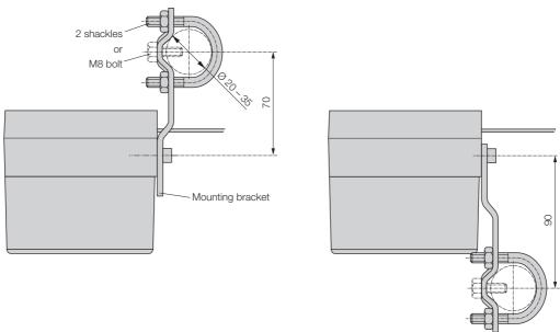
Fig. 9. KINAX SR 709 with fitting recommended by NAMUR.
