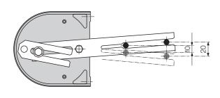
Fig. 3. Operating lever set for minimum operating angle
