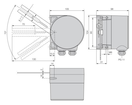
Fig. 8. Position of the KINAX SR 709 operating lever in the upper zero position, corresponding output current 0/4 mA.
