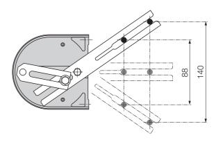
Fig. 4. Operating lever set for maximum operating angle.
