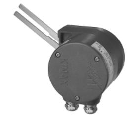
Fig. 2. Position feedback transmitter KINAX SR 709 showing the operating lever in the upper zero position, corresponding output current 0/4 mA.
