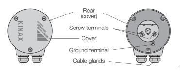
Fig. 5. KINAX SR 709 with screw terminals and cable glands.
